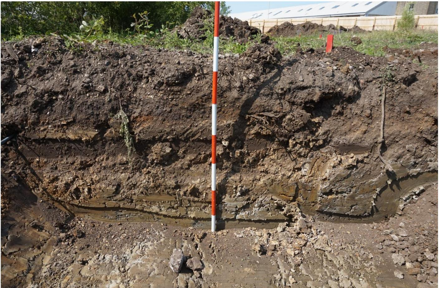
Plate 33: Looking north at section exposed in test pit 4. At the base alluvial clayey loam 405 is overlaid by made ground levelling deposits (404 and 403) followed by railway bedding deposit (402) and sealed with demolition layer 401. The (402) horizon can be seen behind second from the top white section of the scale, Context is rusty brown in colour.
