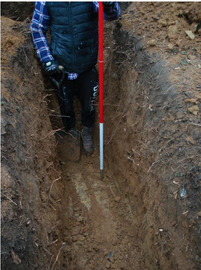
Plate 1. Trial Pit 1. Hard surface of Clay with Flint
