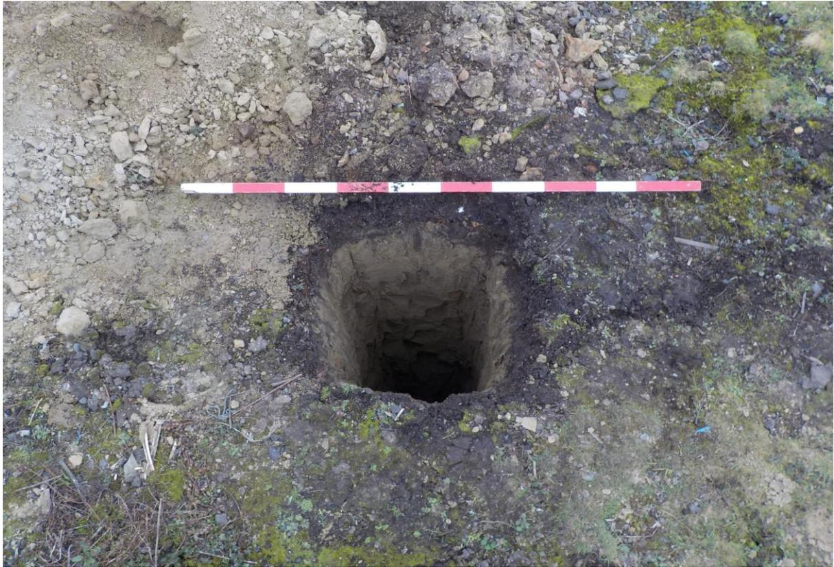
Plate 17: Geological Test-Pit 28. One metre scale bar.
