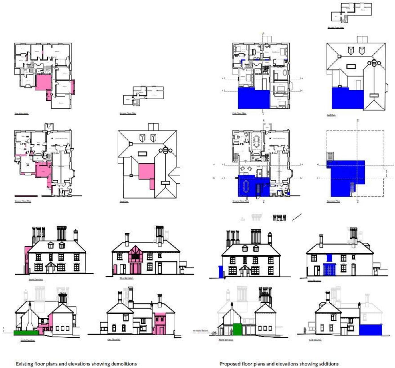
Figure 3. Phases of demolition and proposed build
